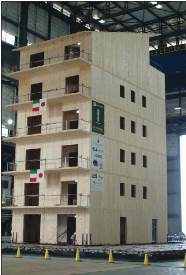
A five-story model building built to demonstrate the use of cross-laminated timbers in multistory residential and commercial structures.
